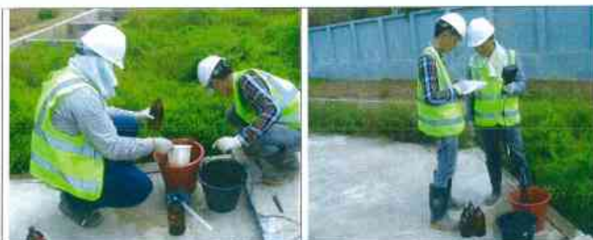
Surface water sampling and onsite measurement at SW-6
