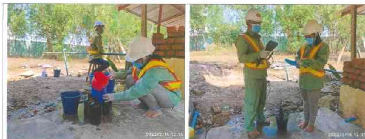
Ground water sampling and onsite measurement at GW-2
