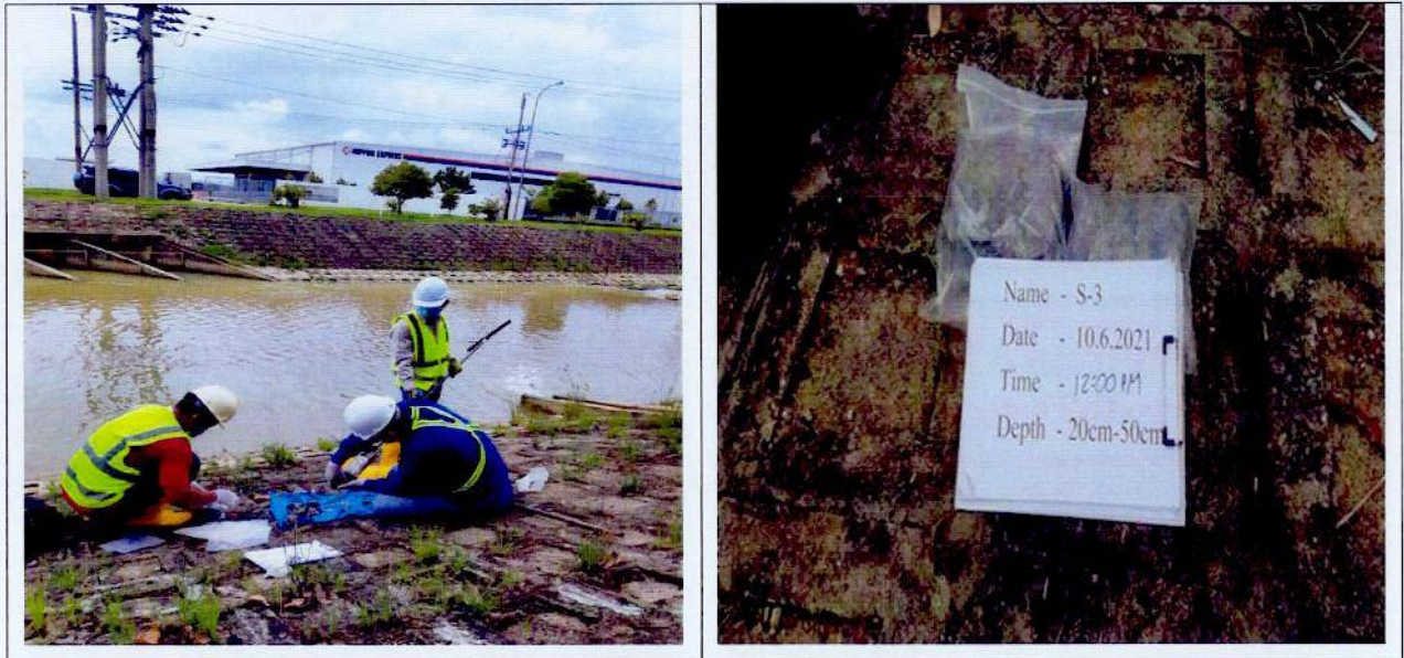
Figure 4 Soil quality sampling at S-3
