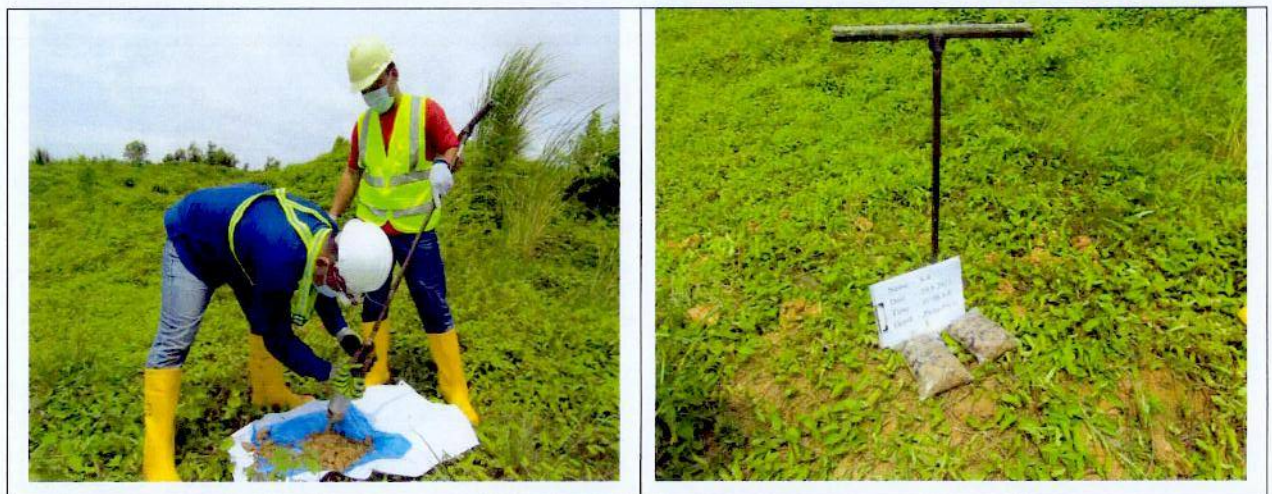
Figure 5 Soil quality sampling at S-4
